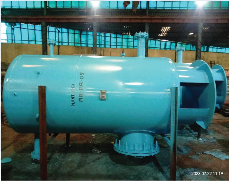
AIR RECEIVER (PLANT AREA)
