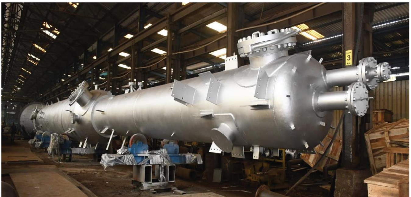
PROCESS COLUMN AT IOCL - 40M LONG
