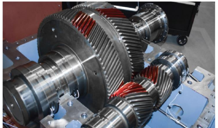
GEAR BOXES FOR UNDERGROUND CONVEYOR
