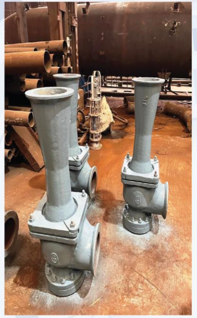
HYDROJECTOR (JET PUMP)
