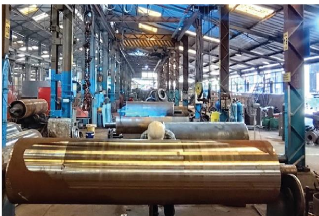
PULLEYS FOR UNDERGROUND CONVEYOR
